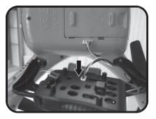
1. Connect the camera cable to the drone with the specified connector.
