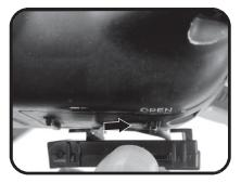
2. Fix the camera in the drone inserting the tabs into the notches.
